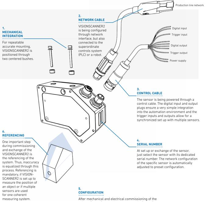
After mechanical and electrical commissioning of the automation environment, measurement tasks can be created. The integrated automation interface can be configured. Now, measuring tasks can be triggered by the superordinate system and measuring and control data can be drawn. Extended feature is the process data interface, which allows for control of the measuring process and specifically the quality of the product being measured.
